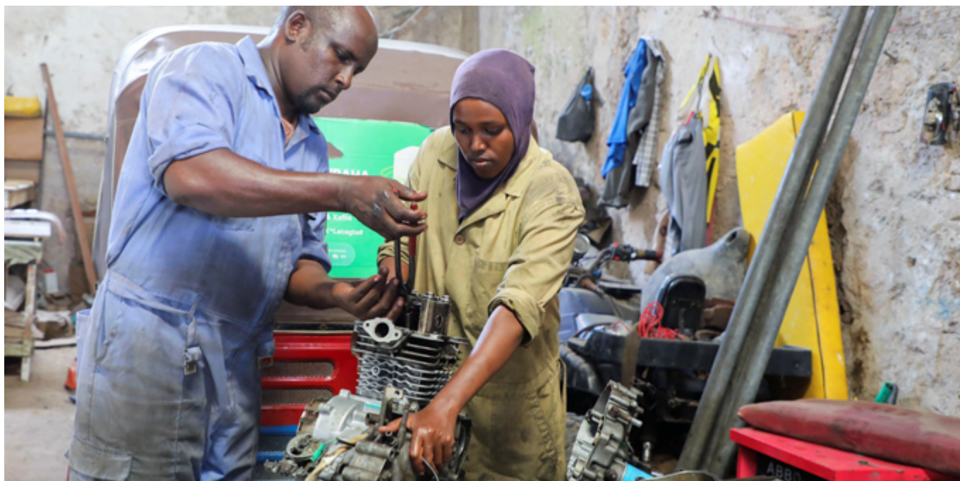
A woman mechanic and her teacher fix the engine of a rickshaw, Somalia. Source: ITF
